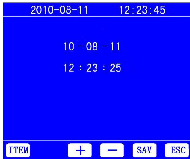
Press the “Item” button to select parameters such as year, month, day, hour, minute, second, press the “Increase”, “Decrease” button to modify the selected parameters such as year, month, day, hour, minute, second, press “Sav” to save after modification, press “Esc” key to return to the boot screen.
