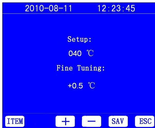
Press the “Item” to select the parameters with the cursor, press the key Tab to select the value of a place of selected parameter, press the “Increase”, “Decrease” to modify the value of a place of selected parameter, Press key “Sav” to save the setting, press “Esc” to return to the boot screen.
