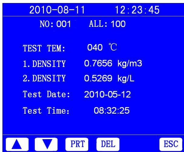
If there is no test record, “No record” shows in the middle of the screen, otherwise the latest one record will be shown. Press “Previous”, “Next” to view
